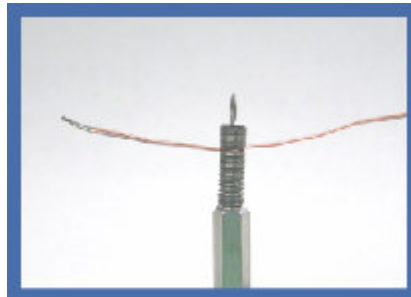
Figure 10. Thermocouple tip between spring coils
